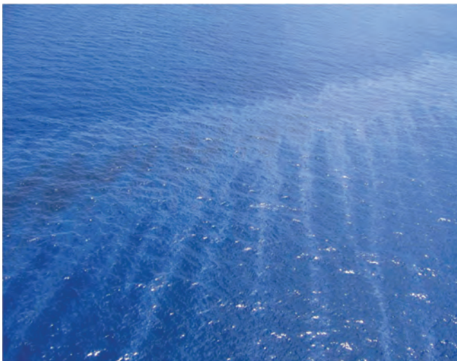
▲ Figure 10: A band of black oil is observed from left to right of the picture. The wind, blowing across the oil, is pushing this band away from the observer resulting in perpendicular windrows of varied sheen.
