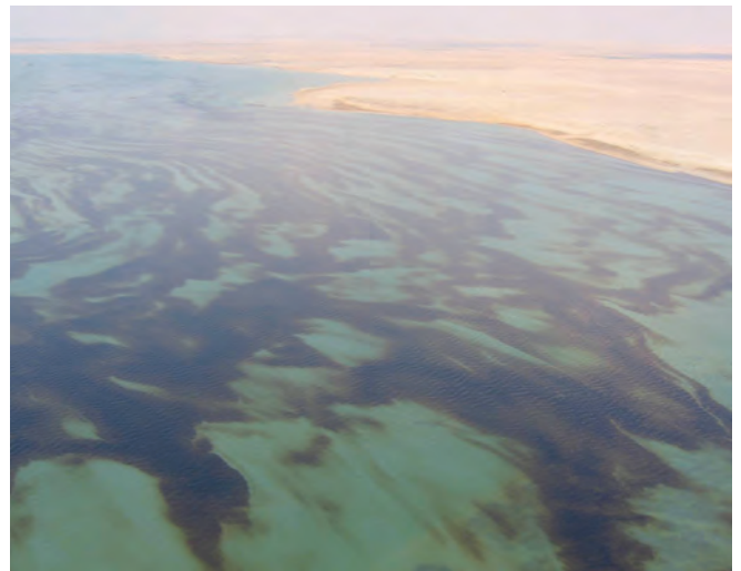
▲ Figure 11: Very large broken slicks of heavy fuel oil - note the absence of sheen.
